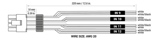
IMPORTANT: with respect to the native 8 SPK IN inputs, the sensitivity scale of the F4IN inputs is 3.2 ÷ 32 VRMS, in order to allow the integration in advanced OEM systems that deliver higher voltages. In the bit Drive software the F4IN input channels will always be #9,#10,#11,#12. Please refer to the following table for a correct sensitivity calibration of each F4IN channel.
