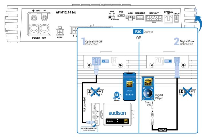
WARNING: the digital input accepts PCM stereo signals up to 192kHz/24bit, therefore it is not possible to play multichannel signals DOLBY DIGITAL (AC3) from audio/video sources (like for example the audio of a DVD movie or DTS). The output of these devices must be configured in STEREO mode to be played.
