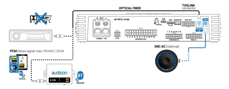
WARNING: the digital input accepts PCM stereo signals up to 192kHz/24bit, therefore it is not possible to play multichannel signals DOLBY DIGITAL (AC3) from audio/video sources (like for example the audio of a DVD movie or DTS). The output of these devices must be configured in STEREO mode to be played.
